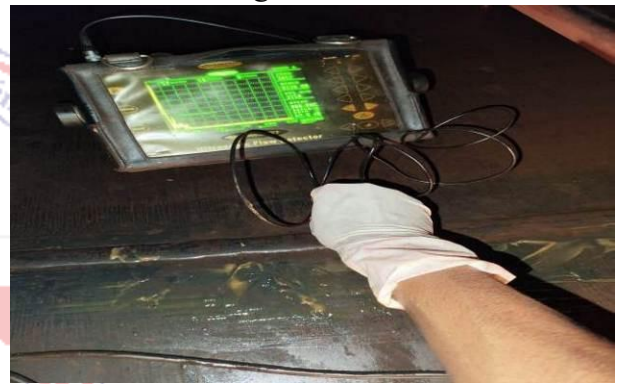
Photo 13: No internal indications were observed in weld joints of vessel in Ultrasonic Testing (UT).
