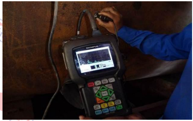
Photo 8: In thickness Measurement, drum thickness found 5.45 mm which was less compare to design thickness of 8 mm.
