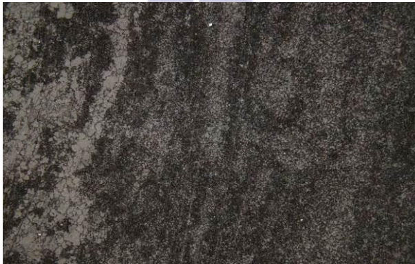
Photo 14: Micro-examination shows recrystallized fine-grained structure of ferrite & pearlite of Heat Affected Zone of weld joint.
