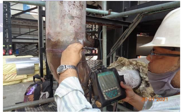
Photo 15: Photographs shows hardness Measurement on outlet pipe of pressure vessel. Reading found with the range.
