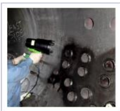
Magnetic Particle Inspection of Boiler Drum
